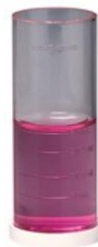
Colourimetric analysis is based on the reaction between  $\text{ClO}_2$  and a dye, and the measurement of the absorbance of a specific wavelength of light after this reaction takes place. The dyes that can be used include N,N-diethyl-p-phenylenediamine (DPD), chlorophenol red (CPR) and Lissamine Green (LGB). Each of these dyes has its own limitations (e.g. the colour of the DPD changes over time, LGB is temperature dependent), but they also have their own positive characteristics.
