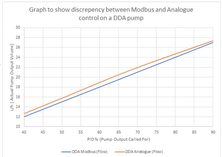
**Graph to show discrepancy between analogue control and Modbus control on a DDA pump - the difference is very small but is measurable. This was measured on a real DDA pump in-house by Pi engineers.**
