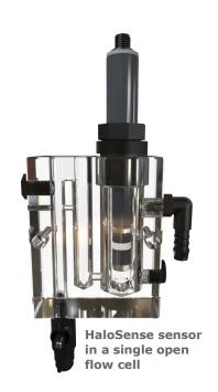
The HaloSense sensor is a three electrode chrono amperometric potentiostatic sensor. The free chlorine molecules diffuse through the membrane and come into contact with the electrolyte.
