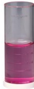
Colourimetric analysis is based on the reaction between  $\text{ClO}_2$  and a dye, and the measurement of the absorbance of a specific wavelength of light after this reaction takes place. The dyes that can be used include N.N-diethyl-p-phenylenediamine (DPD), chlorophenol red (CPR) and Lissamine Green (LGB). Each of these dyes has its own limitations (e.g. the colour of the DPD changes over time, LGB is temperature dependent), but they also have their own positive characteristics.
