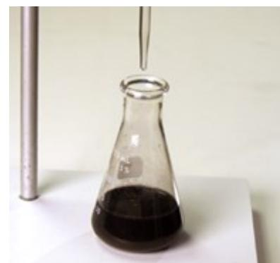
This method relies upon  $\text{ClO}_2$  oxidising iodine ions to iodine, which can then be titrated with sodium thiosulphate. Some relatively simple calculations can then be performed, and the concentration of chlorine dioxide can be deduced.
