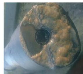
Fig 1: Sensor Fouling
