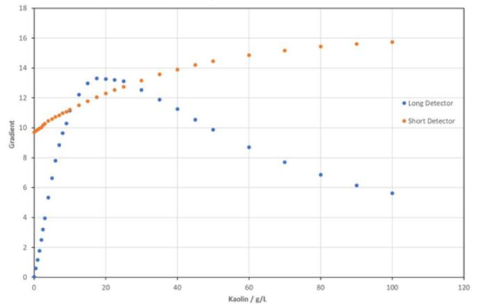
**Fig. 3 Response of a SoliSense<sup>®</sup> sensor to kaolin samples.**
