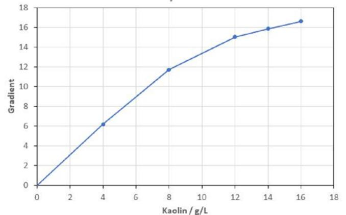
**Fig. 4 Five-point SoliSense<sup>®</sup> calibration graph for kaolin.**
