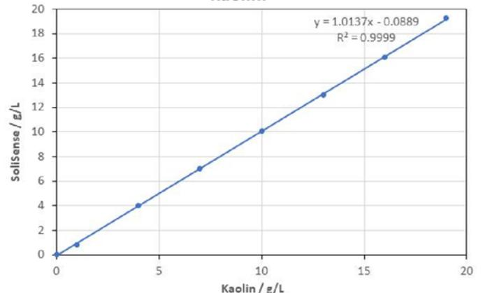
**Fig. 5 SoliSense<sup>®</sup> readings for a range of kaolin samples.**
