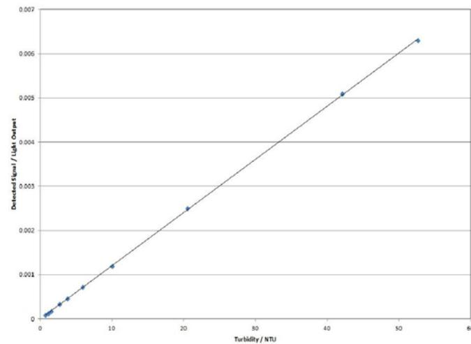
**Fig. 4 Relationship between light emitted/light detected and turbidity.**
