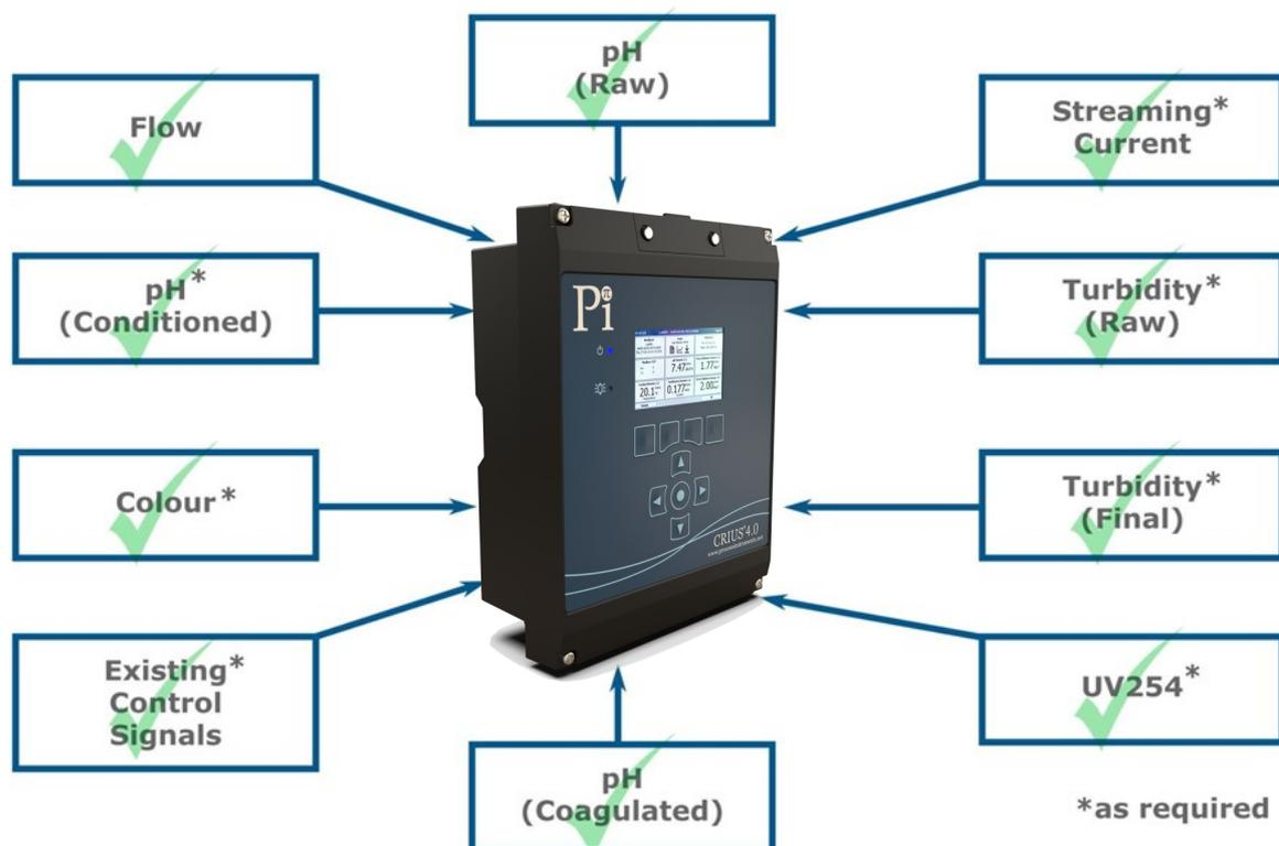
If a plant notices that the Streaming Current is going up and down with pH what they are seeing is that the charge produced by adding the coagulant is being affected by pH changes in the raw water and this would signal that further investigation might be needed to improve coagulation performance. Two things that might be considered are a change in coagulant and/or the introduction of pH control.
