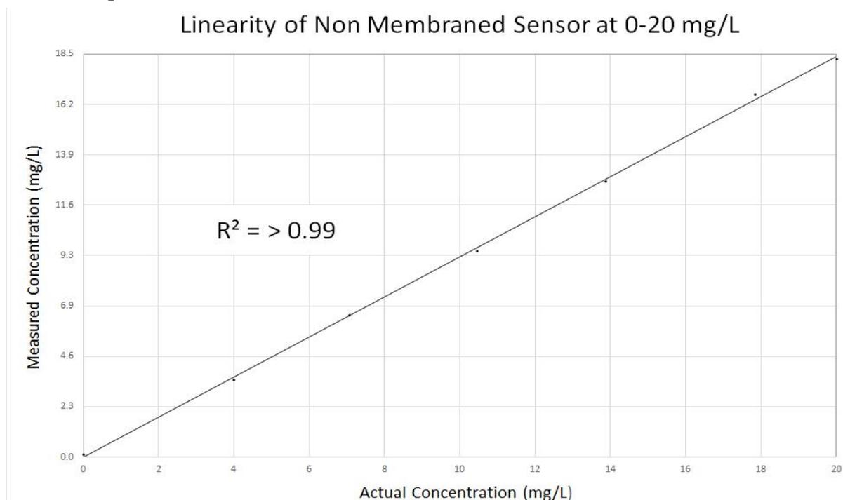
**Fig.2 - A graph showing the linear relationship between the concentration measured by the non membraned sensor and the actual concentration.**
