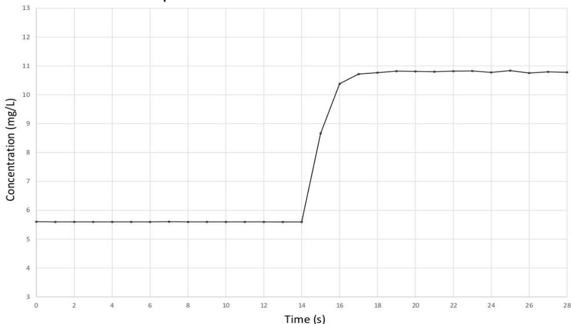
Fig.4 - A graph showing the response time of the non membraned sensor to changes in concentration
